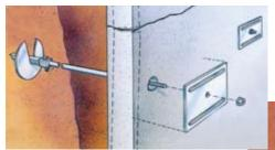
At left, screw anchors tieback retaining and foundation walls.
