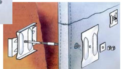
Dura-Grip® Wall Repair System cross plate anchors tieback retaining and foundation walls.
