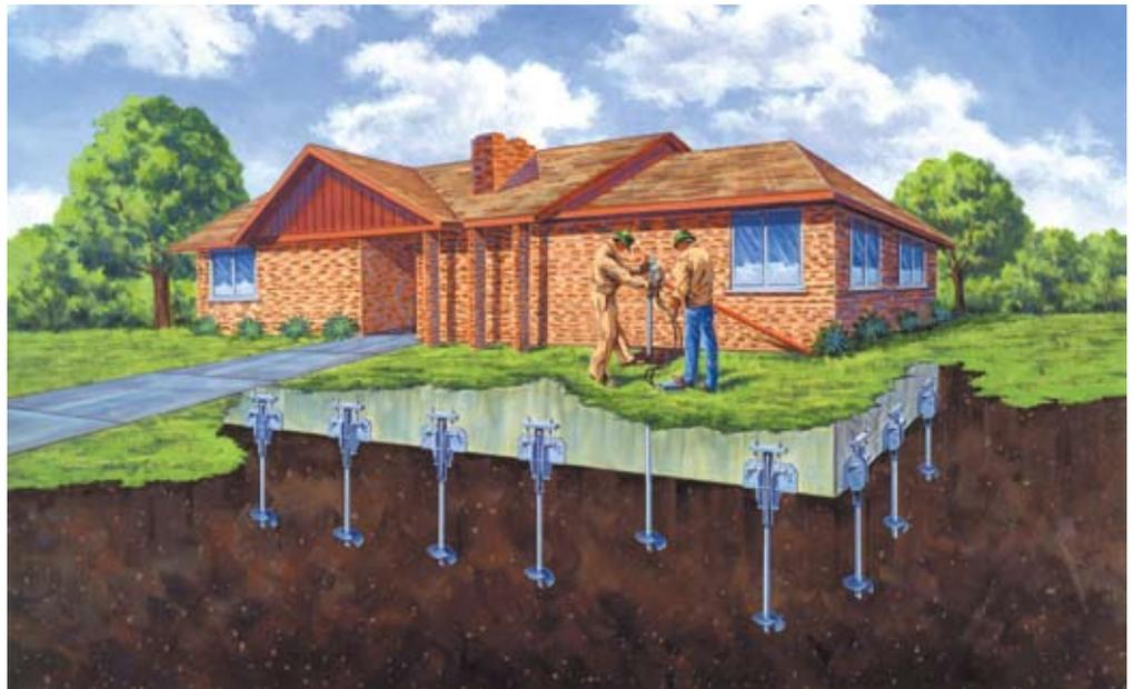
To match individual requirements, helical piles and brackets are selected and spaced at proper intervals to support the loads specific to each home.
